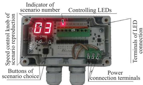
Fig. 1 Purpose of controlling elements and indication
