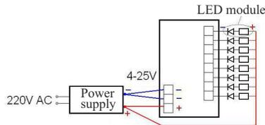
Fig. 2 Scheme of connection of the controller
